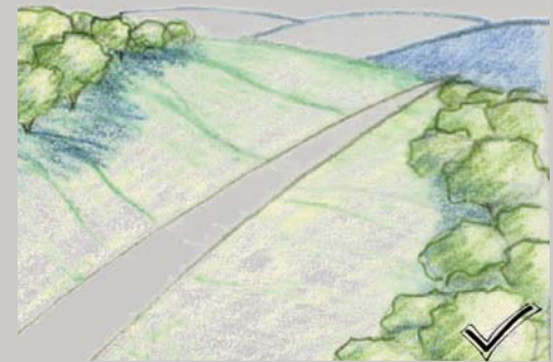
Slope rounding transitions the road back into the natural scenery. The top of cut and toe of fill are invisible.
