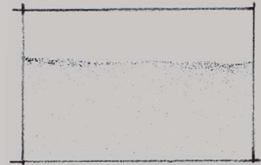
Clay particles are the smallest soil particles. They fit tightly together, which leaves less space for air and water to move through the soil.
