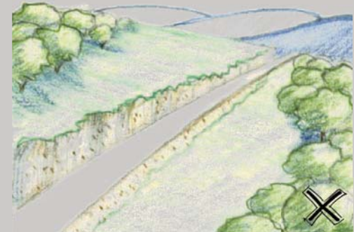
Above, slope rounding was not implemented. Steep cuts and fills erode at the top of the slope. Slope lines are clearly visible.
