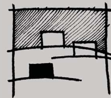
Siting buildings below the horizon lowers their visual impact, and fits them into the landscape.
