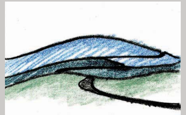
Road alignment along topography minimizing grading.
