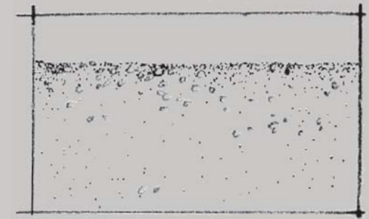
Silt particles are medium-sized soil particles. They allow freer movement of air and water through soil.
