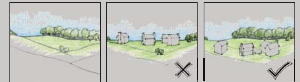
By clustering buildings near the base of the hill, the forest silhouette is preserved.
